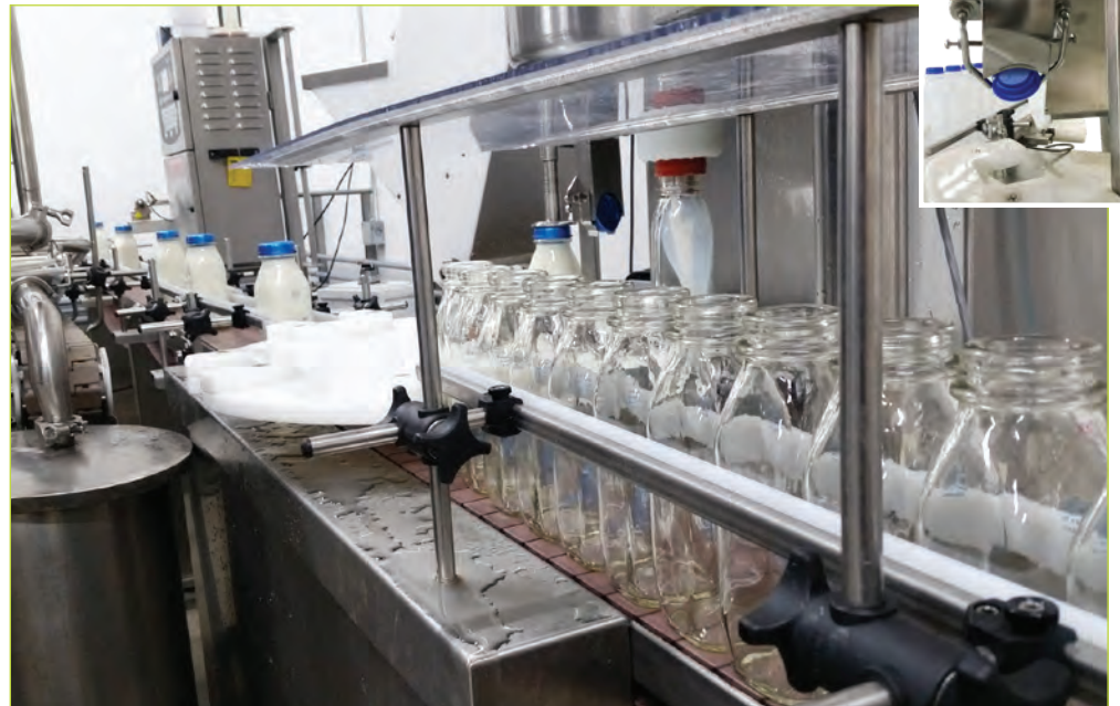
Cap applicator chute on the Automatic Bottle Filler
