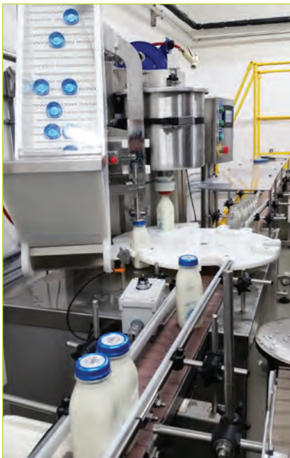
Automatic bottle filler and conveyor line for Stanpac glass bottles at Keystone Pacific
