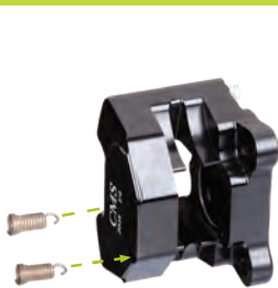
1 Put springs # 5461 into holes in caliper.
