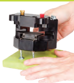
2 Set caliper on assembly tool.
