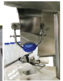
Cap applicator chute on the Automatic Bottle Filler
