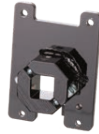
Caliper Bracket w/ Disc Cover Attachment 5342 For 1" and 1 1/8" axle. Powder coated black. Tightens against all 4 sides of the axle, creating less movement caused by vibration.
