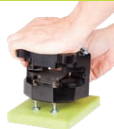
3 Push down on caliper & slide pad in until both springs hook into pad.
