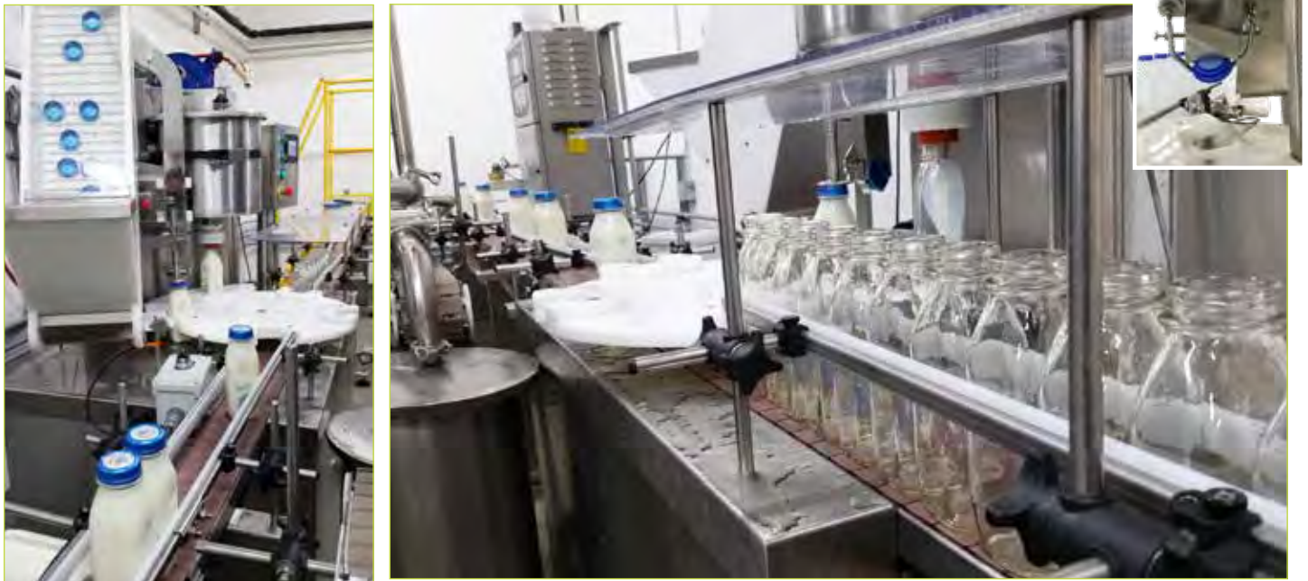
Cap applicator chute on the Automatic Bottle Filler
